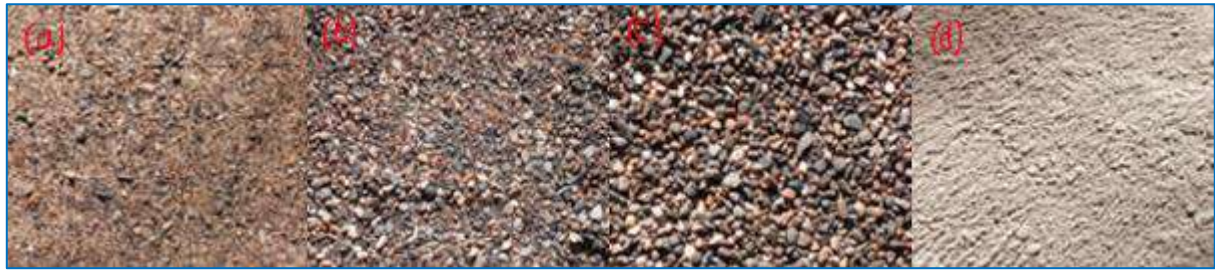
77 78 Figure 1. Test materials: (a) D_{\min} = 0.08 mm; (b) D_{\min} = 0.63 mm; (c) D_{\min} = 2.00 mm; (d) Bentonite.
