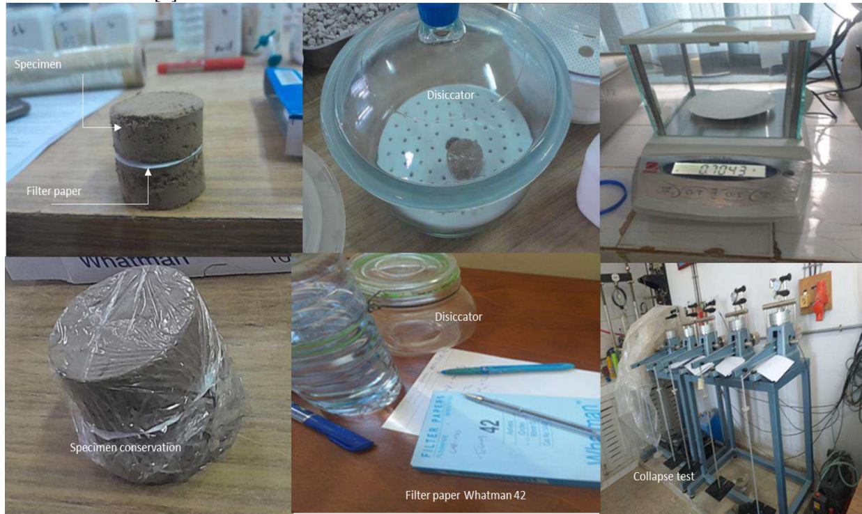
Figure. 2. Experimental procedure for measuring suction using the filter paper and collapse test
